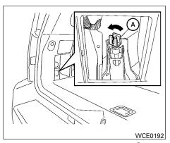
Unscrew the rotating mechanism (A) counterclockwise until loosened on cradle. Remove the jack.
